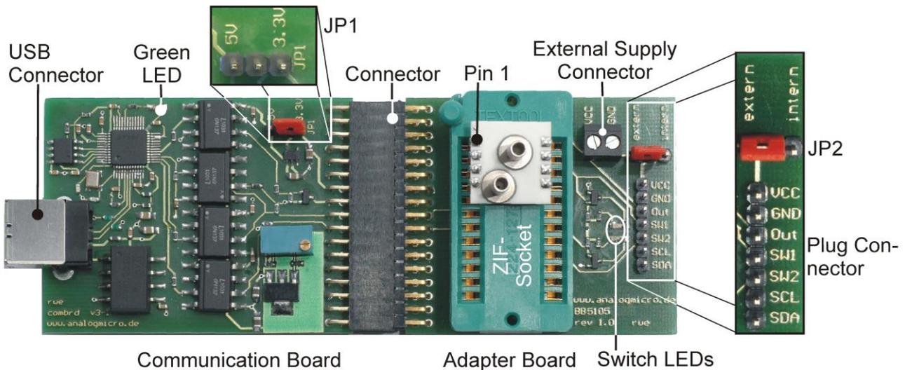
**Figure 1:** USB Starter Kit AMS 5105 with connected sensor.
