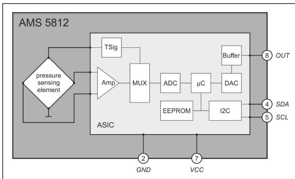
**Figure 1: Functional principle**
