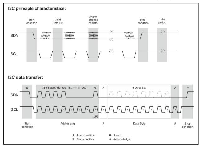
AMS 5812's communication protocol follows a standard I2C communication protocol (see Figure 3)<sup>1</sup>.
