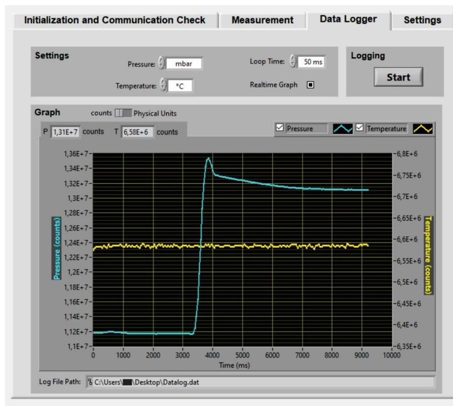
Figure 6: Data Logger Register. The button in the Logging box of the register starts and stops a continuous data measurement. The pressure and temperature measurement values are displayed graphically and saved in a data file.
